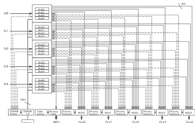
Fig.2. Responsive Link Switch with Packet Overtaking Function
