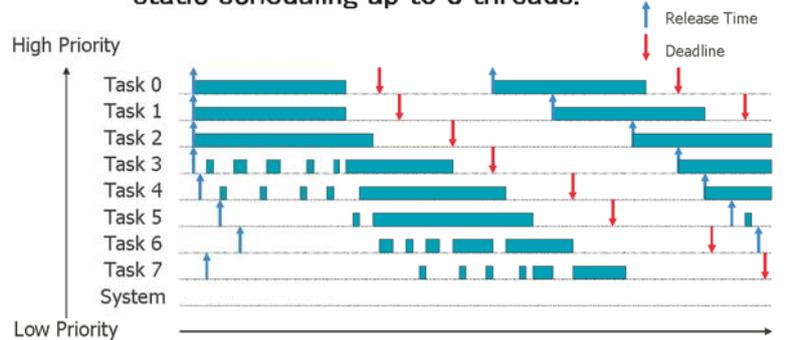
Fig. 8 Real-Time Execution on *RMT Processor*
