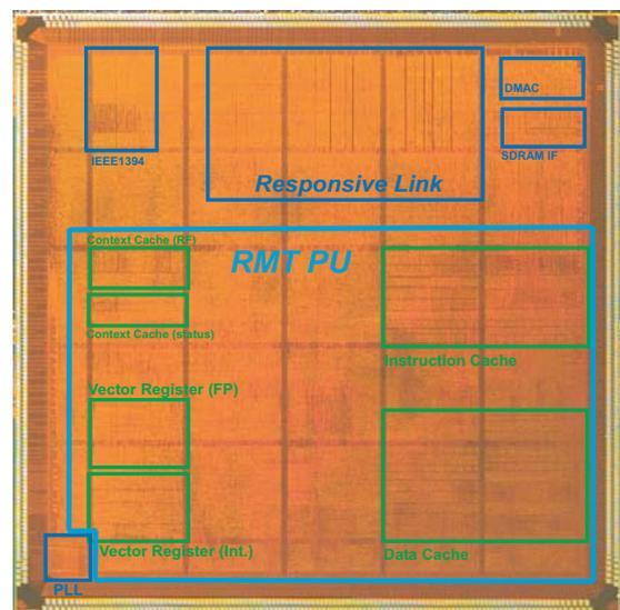
Fig.1 Photo of  $\mu$ RMT Processor**M-RMT Processor design process**
