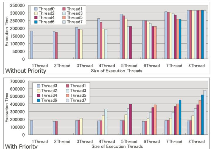
Fig. 7 Execution w/wo Priority on *RMT Processor*
