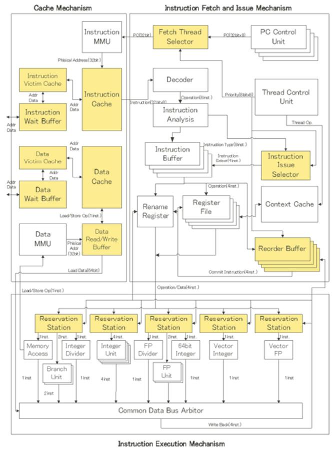
Fig. 4 Block Diagram of *RMT PU*
